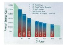
can even be taken straight from the washer-extractor to an ironer or finisher without slowing down the productivity. The high speed, or G-force, is the driving factor. By utilizing the inverter technology it has been possible to achieve this high-speed extraction in freestanding machines. The inverter automatically measures the out-of-balance electronically and decides if the machine can proceed to high speed, generating a high G-force.
